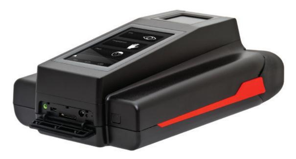
Trident is a completely integrated multi modal mobile biometrics device that combines the world's smallest and fastest FAP 45 fingerprint scanner, the world's first binocular-type iris capture on a mobile device and a stunning five MP auto-focus camera with flash. Trident runs on the latest Android 6.0 OS, widely deployed and proven mobile operating system.
