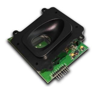
FS83C's fingerprint engine can also extract and match ANSI/ISO template. Please contact Futronic for details.
