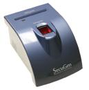
Combination fingerprint reader and contact smart card reader
